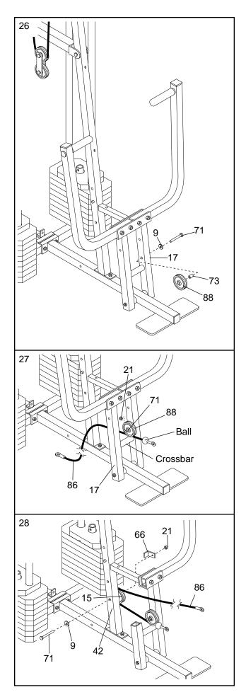
29. Wrap the Low Cable (86) around a 3 1/2" Pulley (15). Attach the Pulley and a Cable Trap (66) to the Press Frame (17) with a 3/8" x 3 1/2" Bolt (16), a 3/8" Washer (9) and a 3/8" Nylon Locknut (21). Be sure that the Cable Trap is turned to hold the Cable in place and that the Cable is routed around the Pulley as shown.
